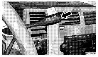
When driving in hilly areas, towing a trailer, carrying a heavy load, etc., and frequent transmission shifting occurs, press the "TOW/HAUL" button. This will improve
